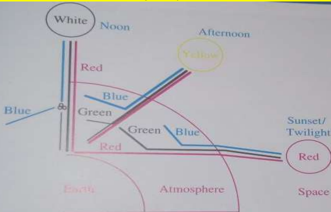
Figure 7.6. Colors of the sun. At noon, the sun appears white because red, green, and some blue light transmit to a viewer's eye. In the afternoon, sunlight traverses a longer path in the atmosphere, removing more blue. At sunset, most green is removed from the line of sight, leaving a red sun. After sunset, the sky appears red due to refraction between space and the atmosphere.
