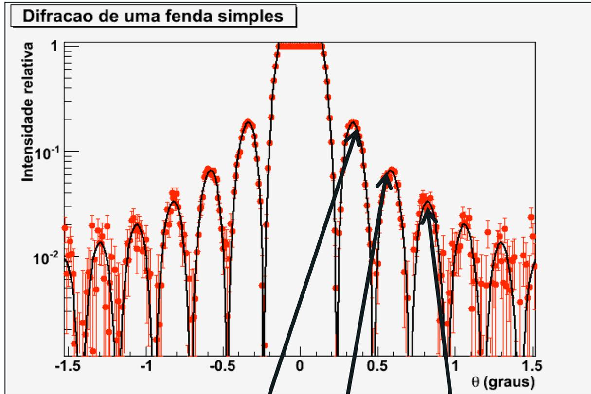
$$I(\theta_{\max}) = \frac{I_0}{\beta^2} = \frac{1}{(2m+1)^2} \frac{4I_0}{\pi^2} = 1 \frac{4I_0}{\pi^2}, \frac{1}{9} \frac{4I_0}{\pi^2}, \frac{1}{25} \frac{4I_0}{\pi^2}, \dots$$
