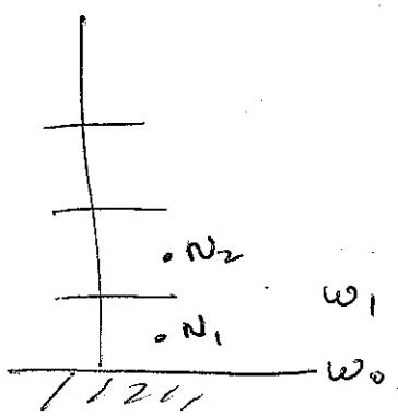
$$\left\{ \begin{array}{l} N_{t+1}^K = N_t^K - \frac{\Delta t}{\Delta z} (F_K - F_{K-1}) \quad (1 \leq K < M) \\ N_{t+1}^1 = N_t^1 - \frac{\Delta t}{\Delta z} (F_1 - F_{fc}) \quad K=1 \\ N_{t+1}^M = N_t^M - \frac{\Delta t}{\Delta z} (F_{top} - F_{M-1}) \quad K=M \end{array} \right.$$
