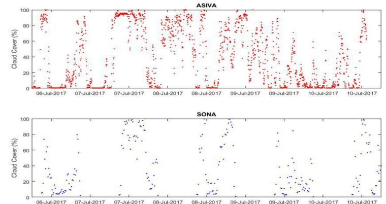
Comparison of cloud cover (%) measured with our instrument (below) and the All Sky Infrared Visible Analyzer (ASIVA, top).
