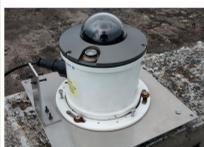
The skyimager consists of a regular digital camera, inside a metal housing with a fisheye lens attached on it. The camera used is a Blackfly 20E4-color, manufactured by point grey. The resolution is 1600x1200.
