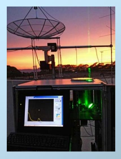
Elastic-backscatter lidar: Nd:Yag - Quantel CFR 200 20 mJ @ 532 nm Pulse: 8 ns, Rate: 10 Hz Divergence: 0.5 mrad
